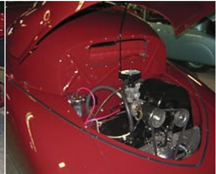
Air-cooled boxer-4 mounted in the rear.
